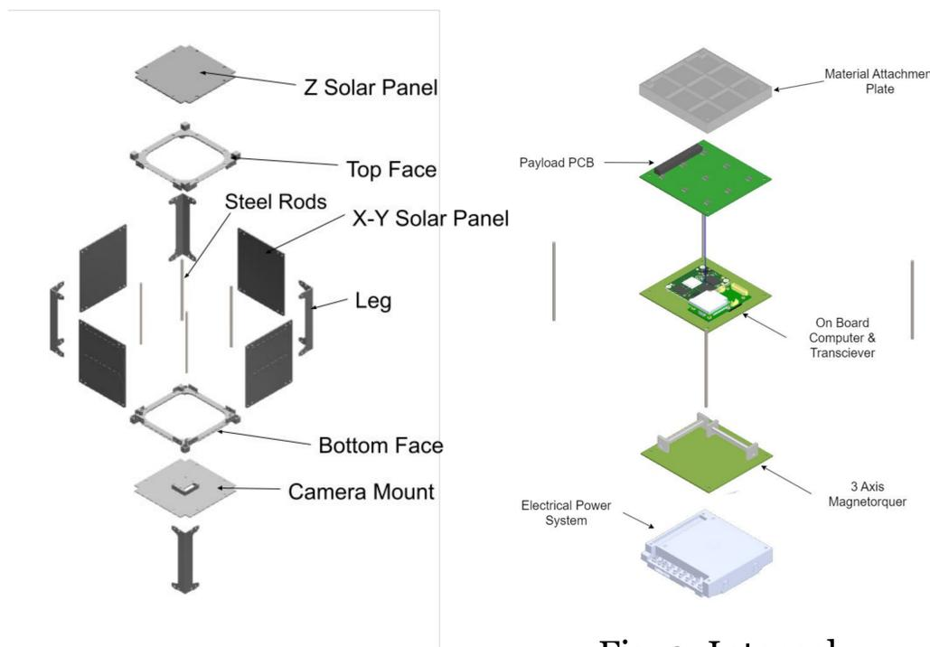
Fig. 2: ROSIsat Chassis Exploded View
