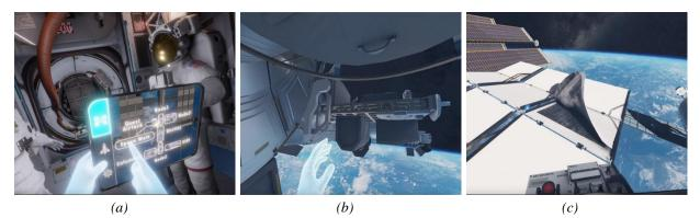
*Note.* Photos depict (a) decision menu selection, (b) handrail (virtual) navigation to the site, and (c) physical (virtual) inspection of anomaly (damaged radiator panel). From "*Mission ISS*" by Magnopus, 2017 (https://www.magnopus.com/mission-iss). Copyright 2017 by Oculus VR LLC.
