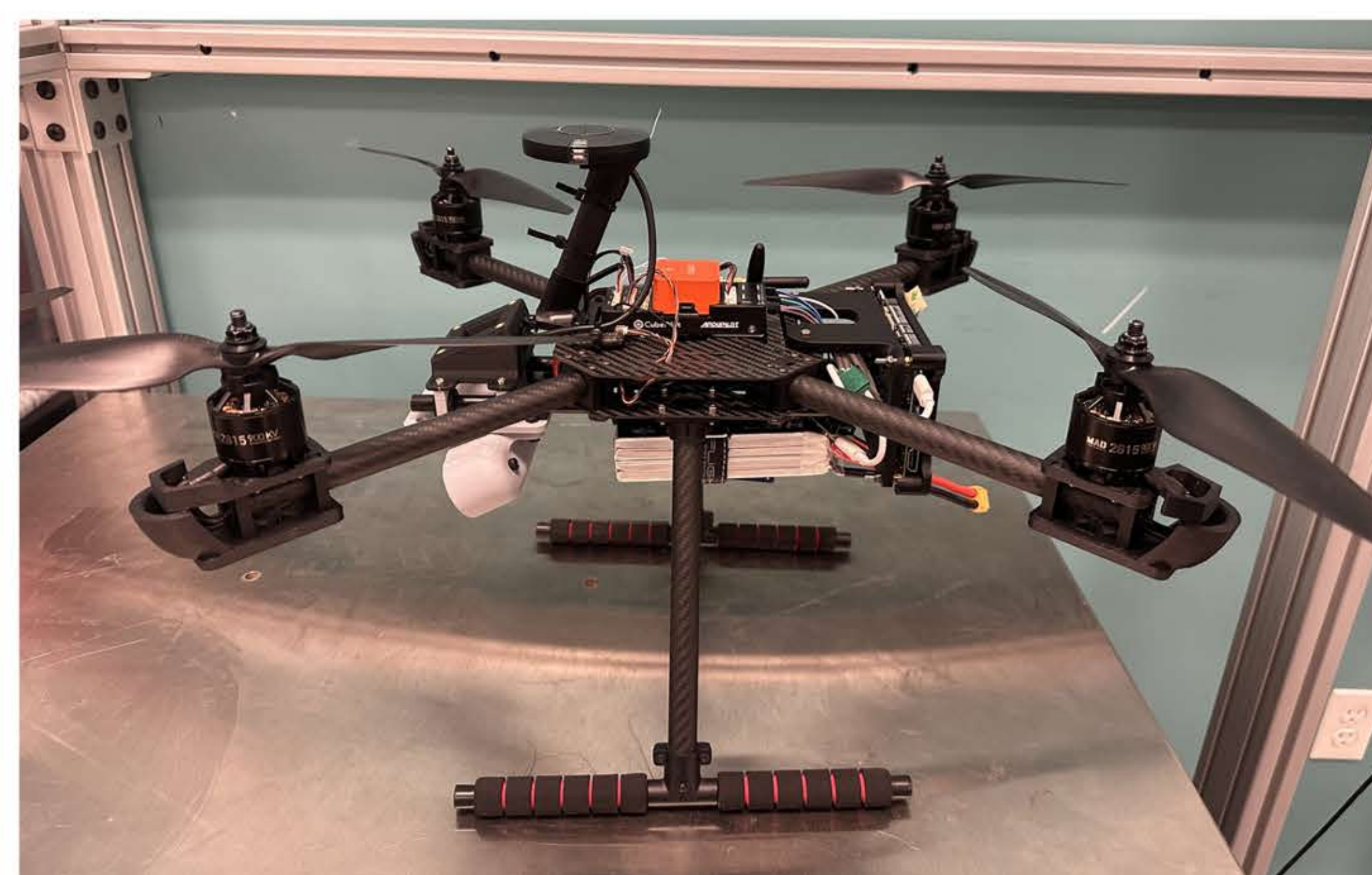
Figure 1: UAS with camera and companion computer
