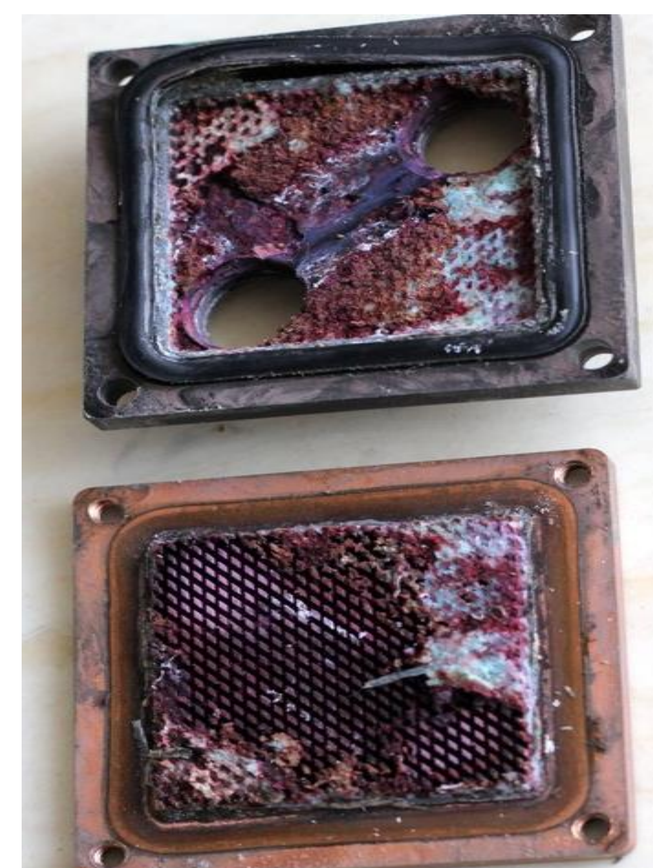
Fig. 6 Corrosive Internal Buildup of Component Parts in a Computer Cooling System
