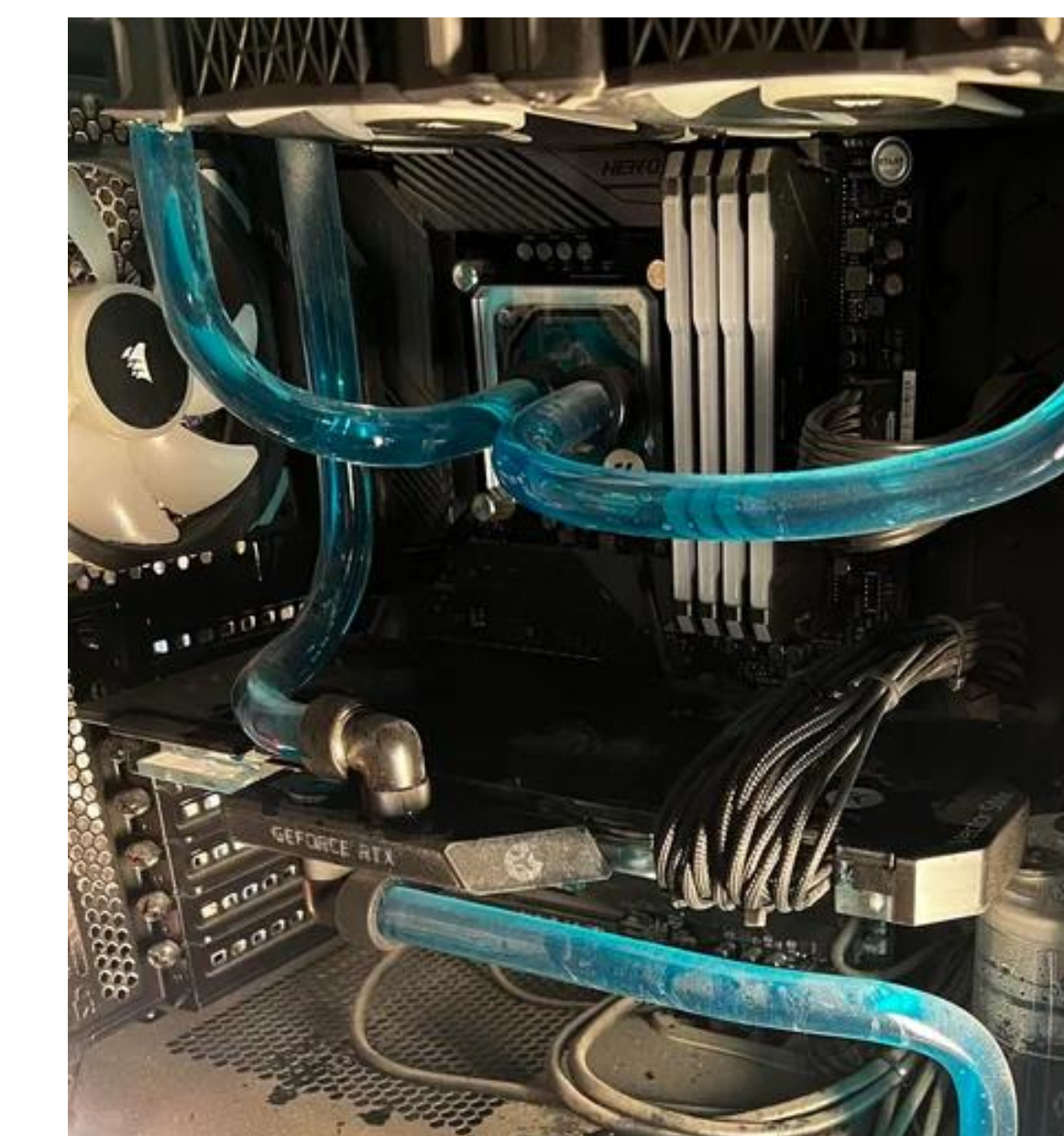
Fig. 8 Water Cooling Server System Leak
