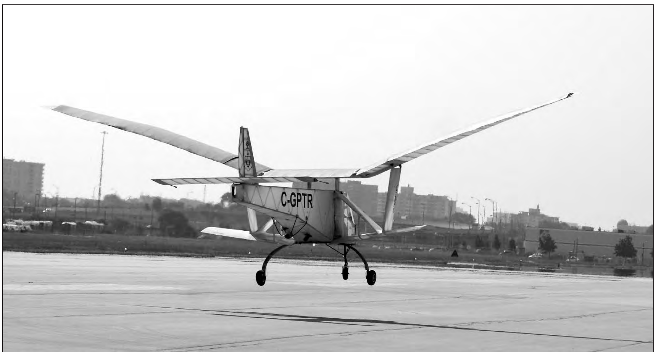
FOR THE FIRST TIME in history an ornithopter successfully flew and sustained powered flight for a third of a kilometer and 14 seconds. The jet powered "Flapper" achieved flight by flapping its wings similar to birds.
