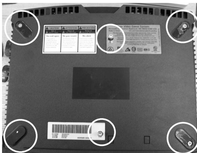
Figure 1. Xbox screw locations.
