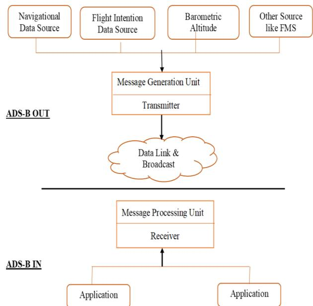
Fig.1. Design of ADS-B System (FAA, 2017, a)
