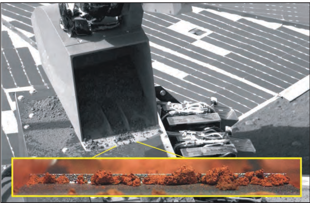
THE ROBOTIC ARM ON Phoenix empties a soil sample into the wet chemistry lab to look for life. It confirmed theories of water-ice and life supporting nutrients in the Martian soil.
