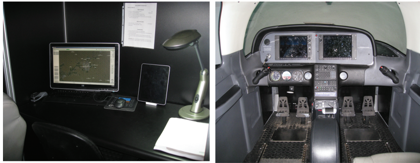
Figure 1. Instructor station (left) and the Cirrus SR20 AATD.
