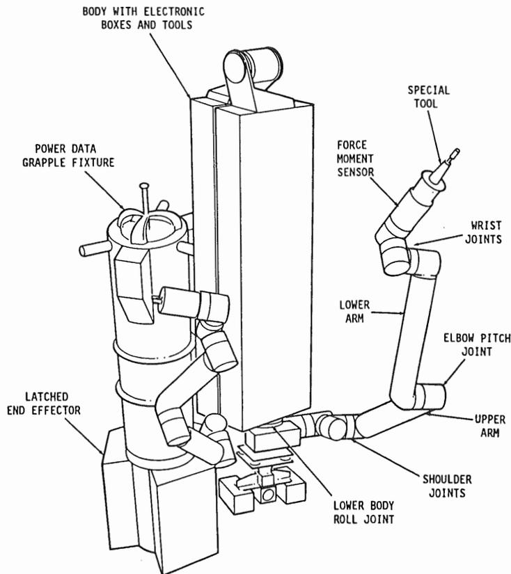
FIGURE 4-4 SPDM CONFIGURATION
