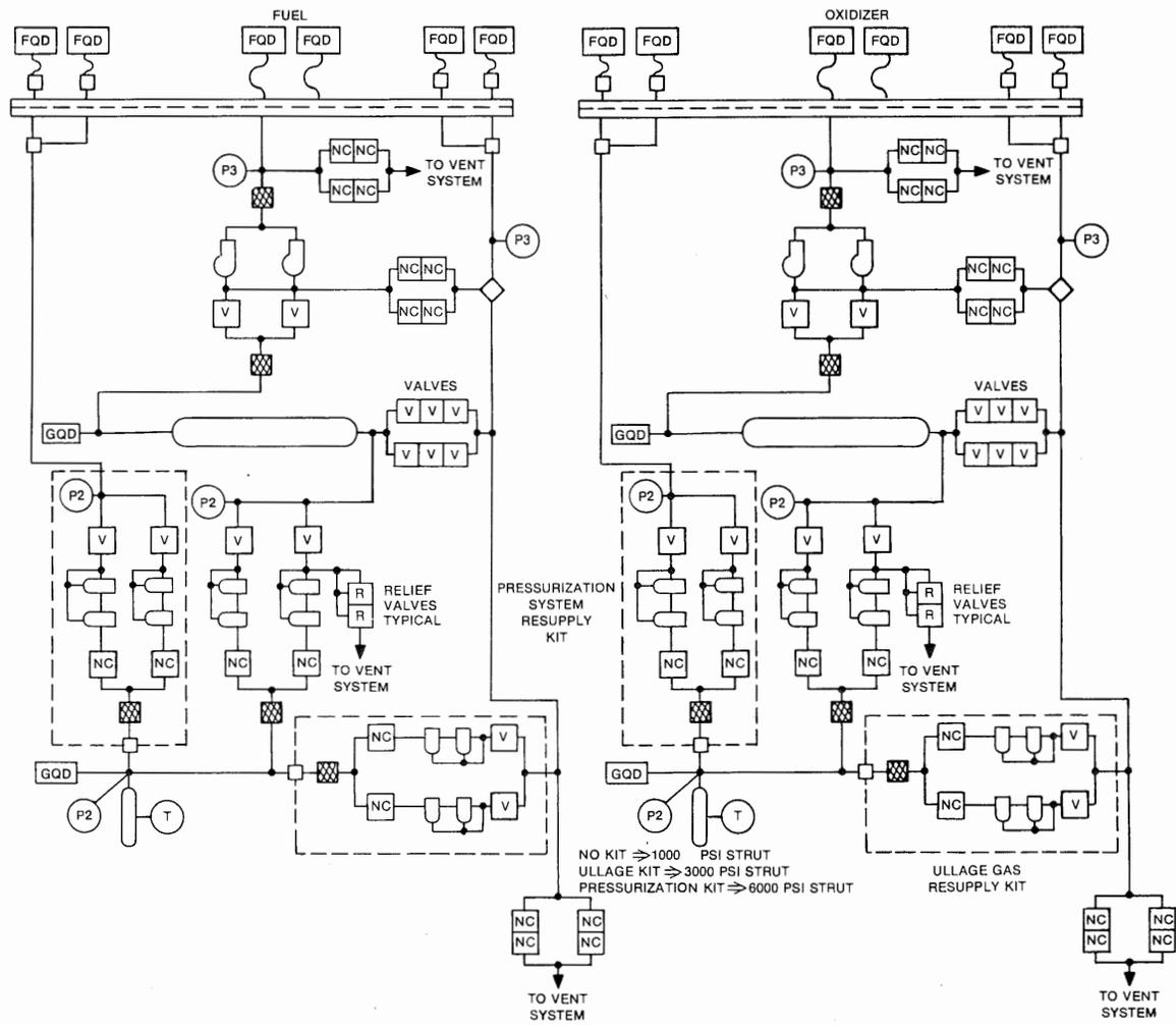
Figure 8. Bipropellant Fluid Subsystem Schematic
