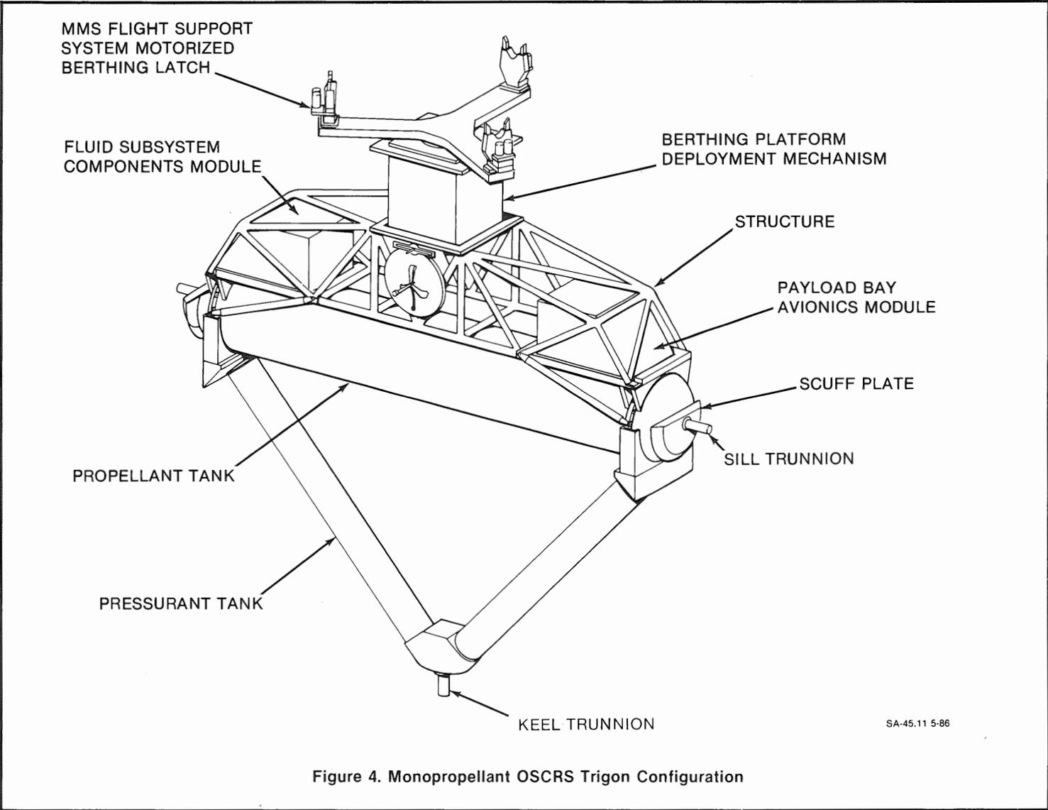
Figure 4. Monopropellant OSCRS Trigon Configuration
