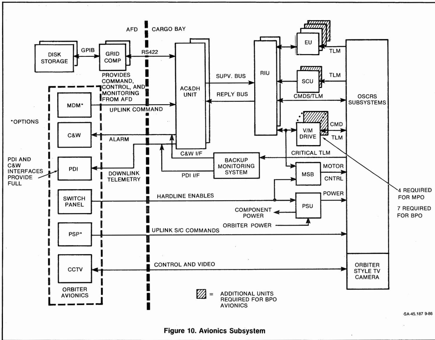
Figure 10. Avionics Subsystem
