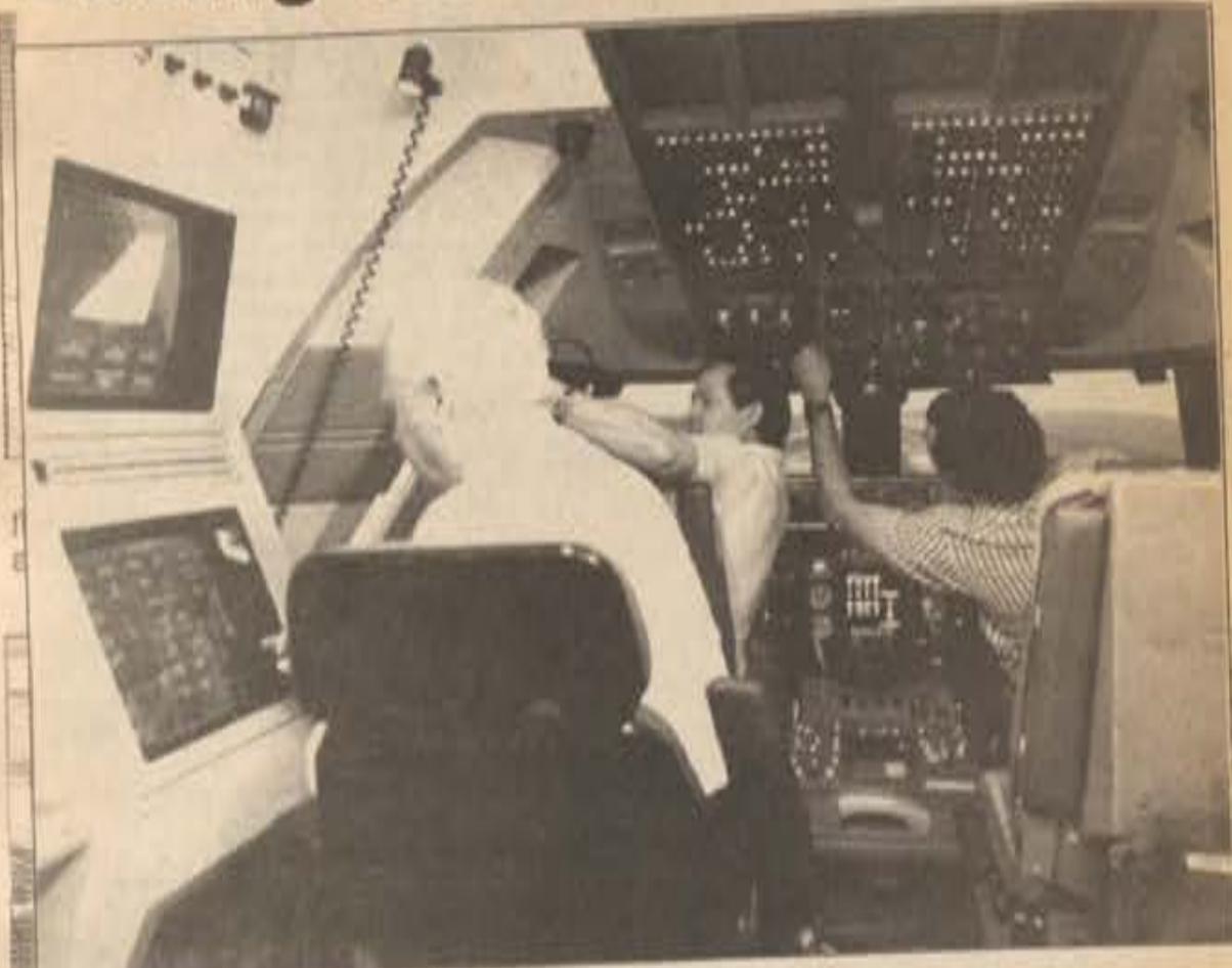
Training taken to new heights... Ed Hoyt instructs two commercial airline pilots in a 747-400 flight simulator. A computer generates realistic images and full motion to provide pilots with what they would actually undergo in a real life situation.
