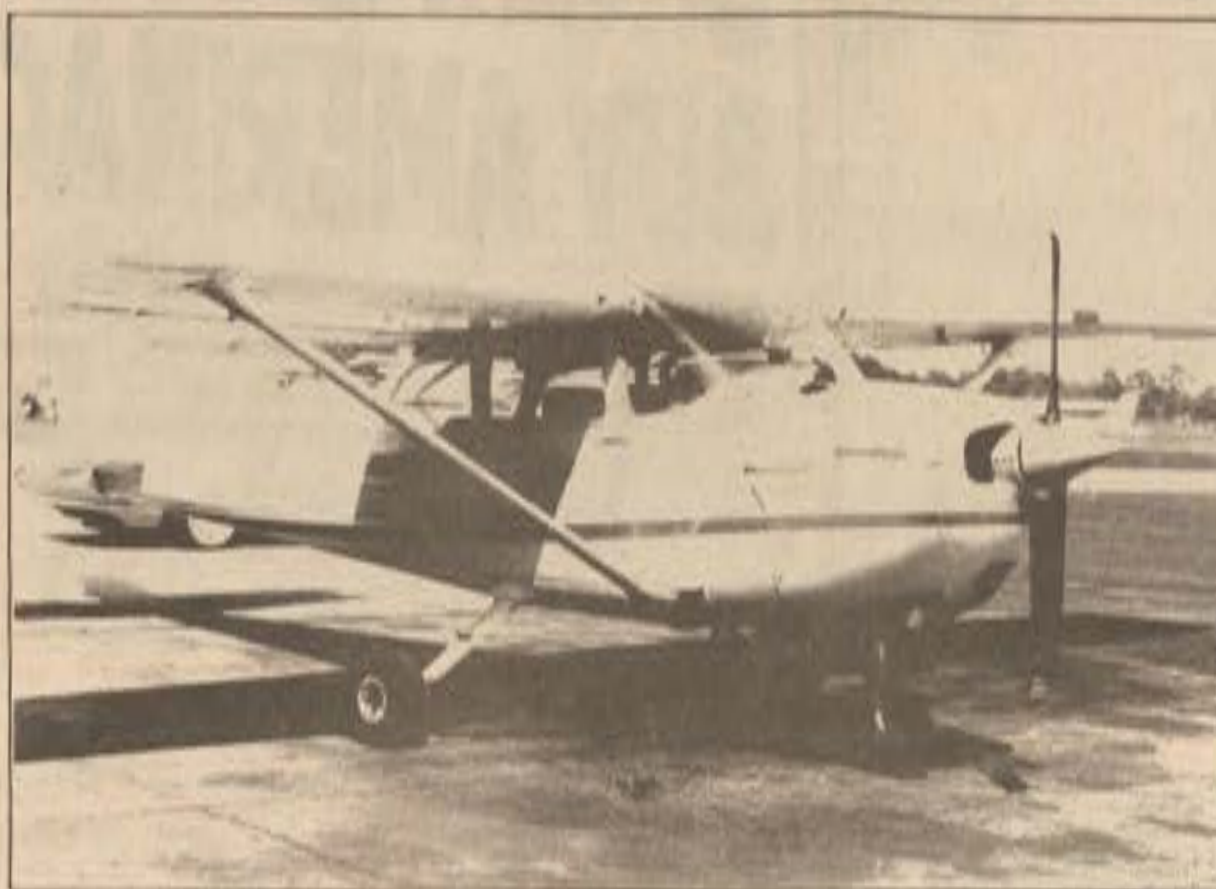
This C-172 was damaged as a gust brought the propeller into contact with the ground.
