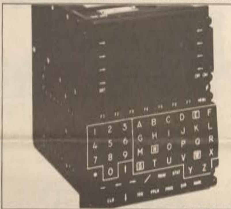
The Collins Control Display Navigation Unit is a panel mounted display with dedicated keys and a full alphanumeric keyboard. The system will be installed on 23 different Naval aircraft.
