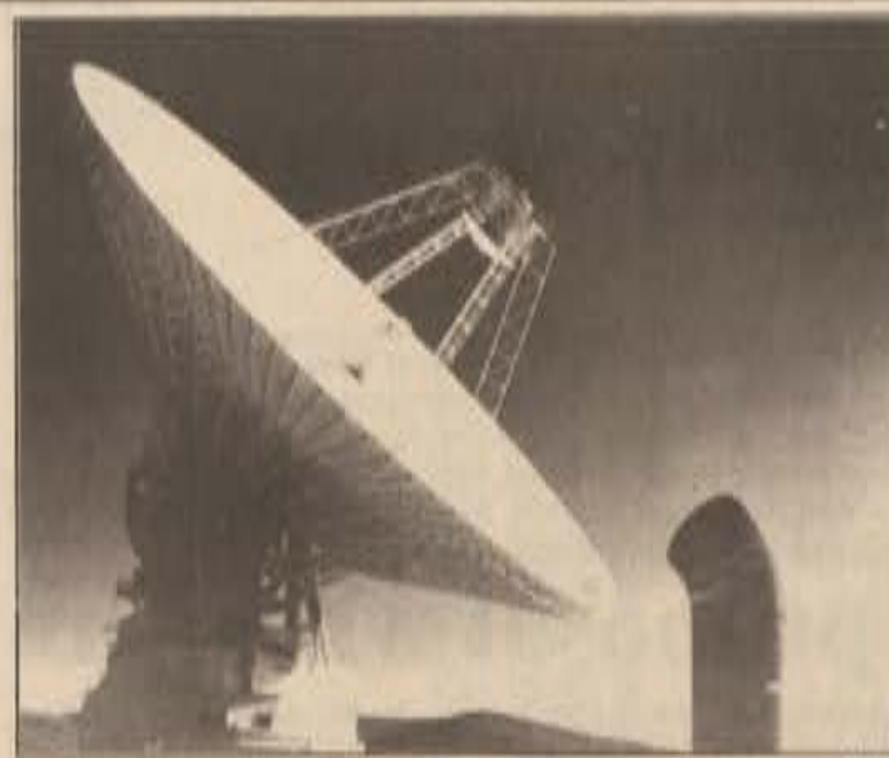
This 70-meter antenna at Goldstone and two other stations around the world keep communications open to satellites and probes throughout the universe.
