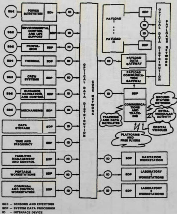
Figure 1. Space Station DMS Reference Configuration
