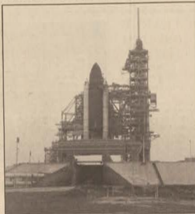
The orbiter Columbia, attached behind the external tank and solid rocket boosters, sits on pad 39A. The three main engine turbopumps have been replaced with new ones and the launch is now back on track.
