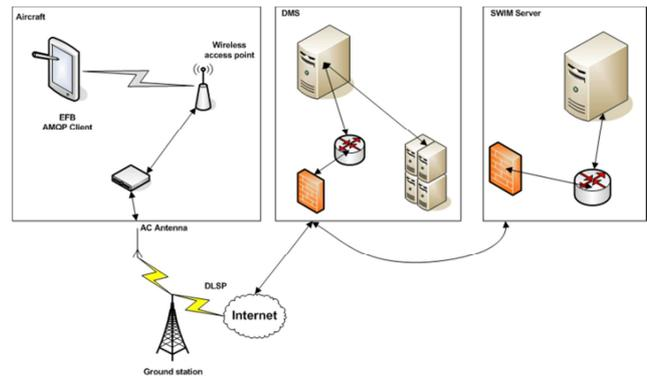
Figure 2. EFB Physical Connectivity Layout
