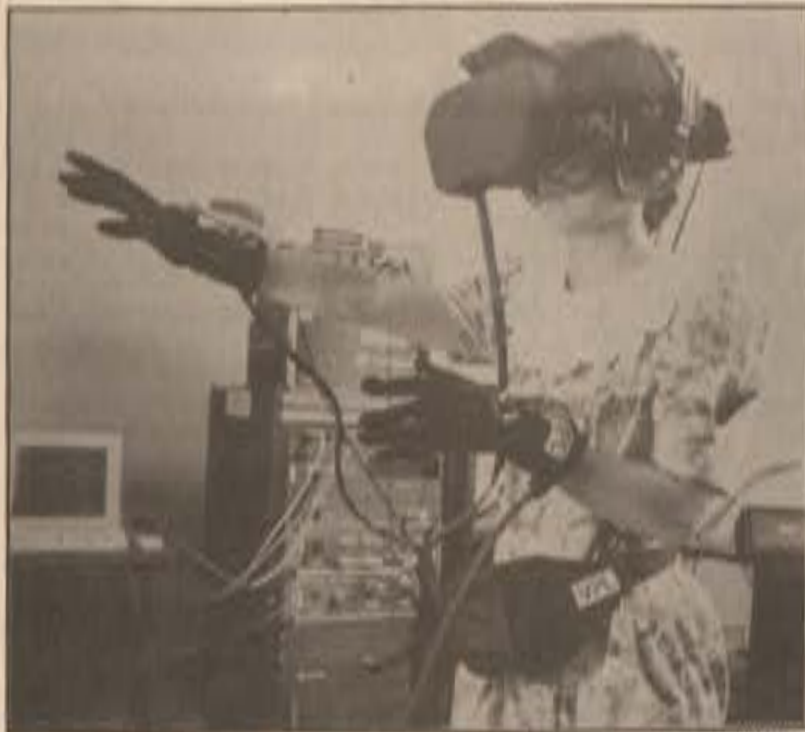
A member of the programming team that designed the virtual reality software tests the headset and gloves for fit and comfort. The astronauts who are scheduled to perform extravehicular activities to repair the Hubble Space Telescope have been training with this equipment.
