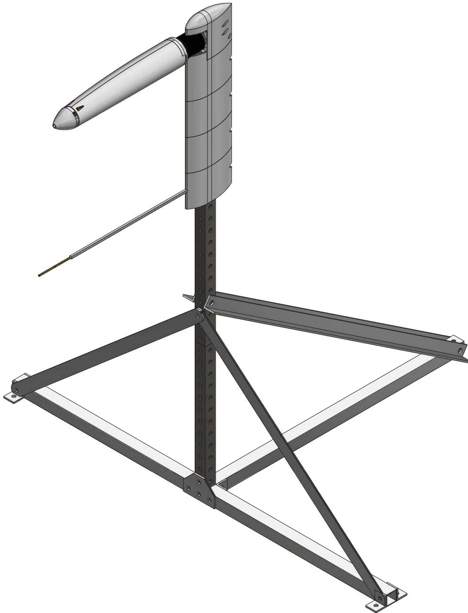
Figure 5: An isometric CAD rendering of the propulsion system testing apparatus with the automotive platform mount and pitot-static probe.
