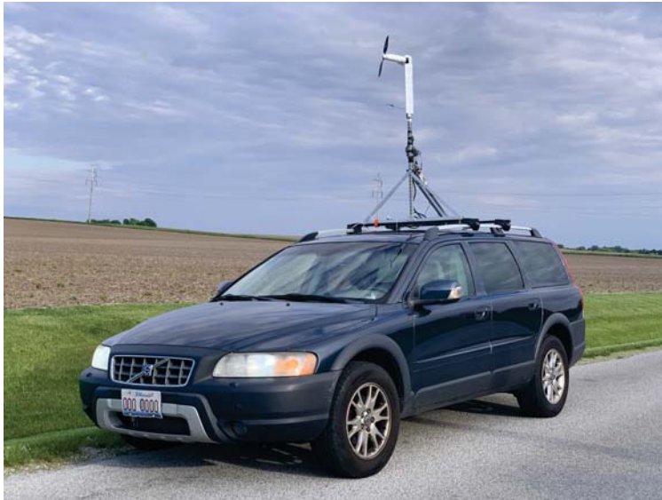
Figure 11: A photo of the propulsion system testing apparatus mounted atop a car for validation testing.
