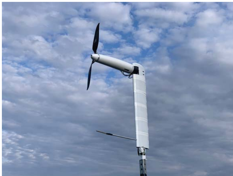
Figure 2: A photo of the propulsion system testing apparatus with folding propeller and pitot-static probe.
