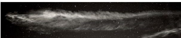
Figure 2. Example of TMA trail about thirty minutes after release showing potential signs of stratified turbulence. Photo from 2012 ATREX campaign launched from Wallops Island, Virginia.
