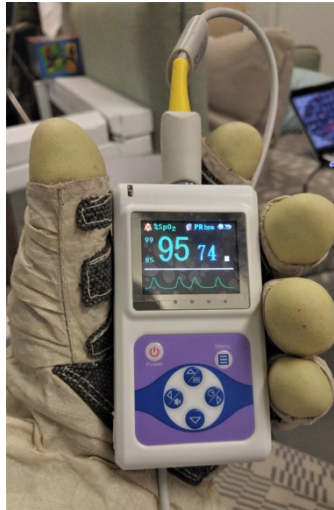
Figure 3: blood oximeter worn under the TMG glove for EVA 4. The tethered recorder was in a pocket within the spacesuit.
