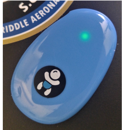
Figure 4: Wearable skin temperature sensor used on all MDRS Crew 188 EVAs under the left armpit.
