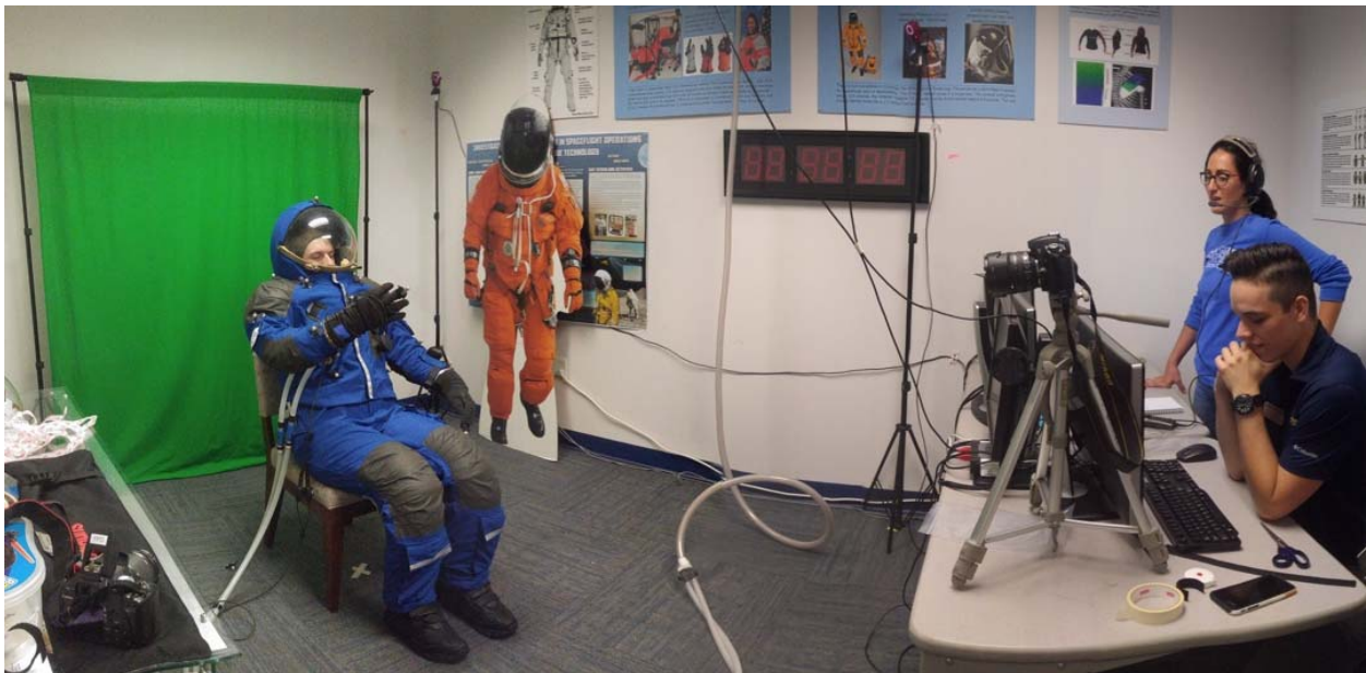
Figure 1. The original S.U.I.T. Lab location as seen in November 2017 for the FFD FOP testing. Four cameras are set up on tripods around the test subject with Peyton Schwartz as test director on a communications loop, Chase Covello as the motion capture recording technician, Ryan Kobrick recording video and taking photos, and Ted Southern as the primary spacesuit technician and safety officer.
