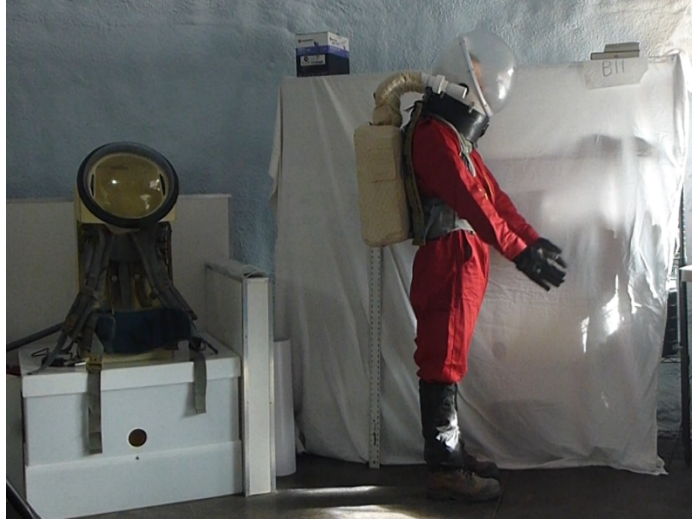
Figure 8: MDRS Crew 188 test subject carrying out ROM Task B11 in SUIT 1. SUIT 2 PLSS is seen on left shelf.
