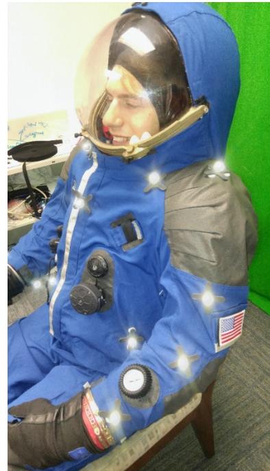
Figure 7: Spaceflight Operations ERAU undergraduate student participating as a test subject in S.U.I.T. Lab ROM test with FFD's NASA FOP spacesuit.
