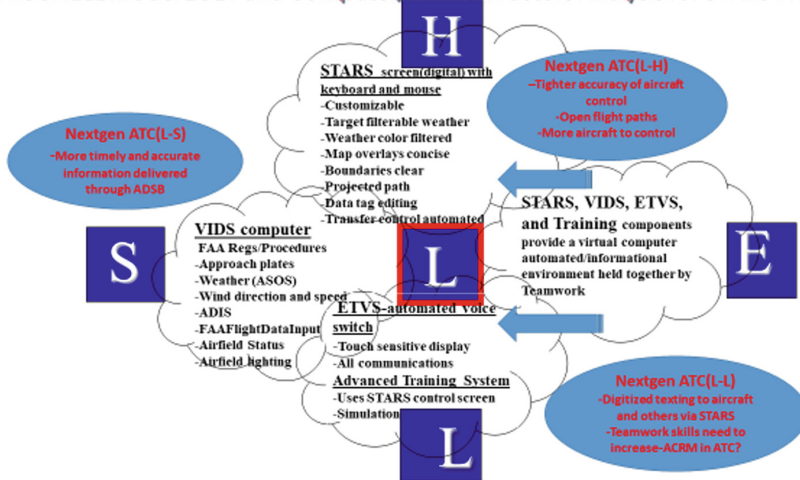
Fig. 2. The SHELL model 2017 adopted for the computer-automation/information of the STARS TRACON controller with predicted Nextgen ATC effects by Mark Miller in 2019.
