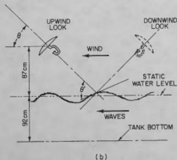
Figure 3 - Two-scale scattering geometry.
