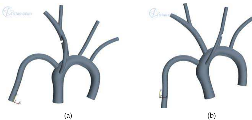
Fig. 10. Solid model of adult aortic arch with LVAD conduit at normal angle of incidence and (a) aortic-to-innominate (IA) bypass and (b) aortic-to-left-carotid (LCA) bypass
