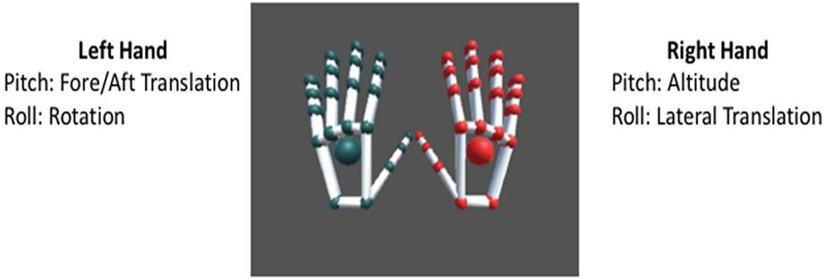
**Fig. 4.** Leap motion UI for controlling camera view
