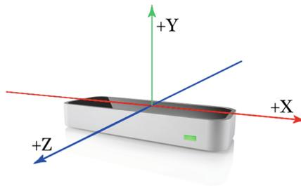
**Fig. 3.** Leap motion controller and coordinate system [13]
