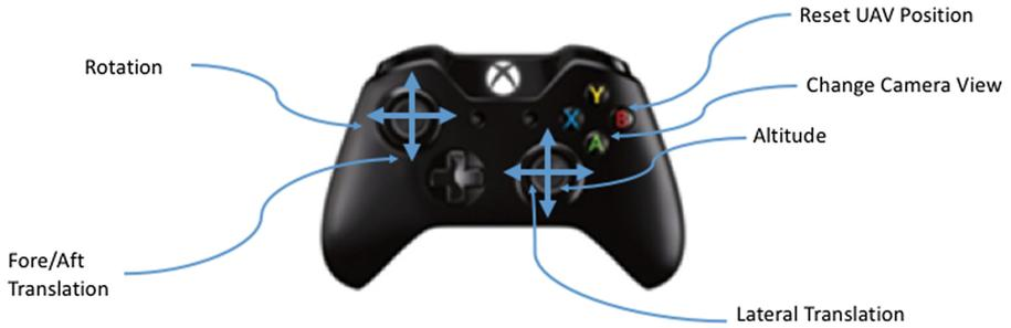
**Fig. 2.** Joystick controller
