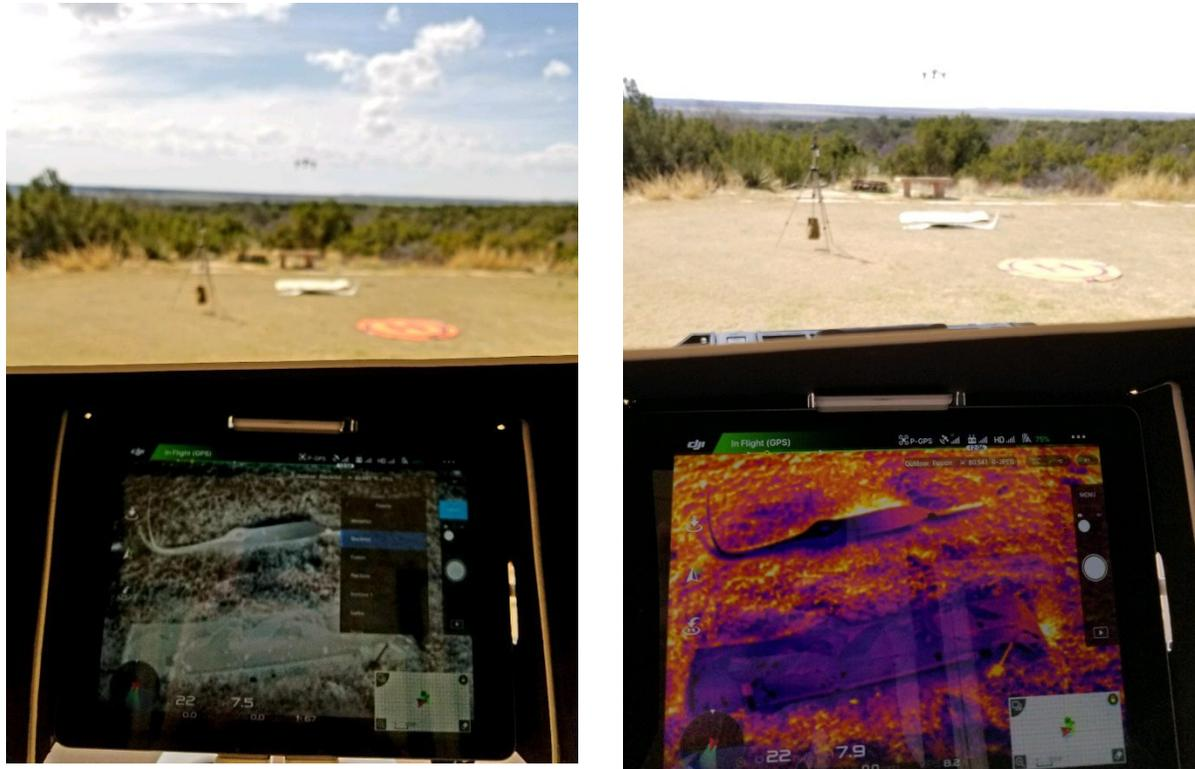
Figure 5. sUAS tablet display of real-time sensor data while the vehicle is in flight.
