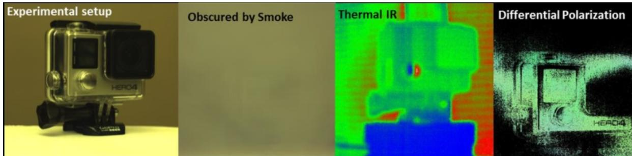
Figure 16. ERAU imaging through fog simulation
