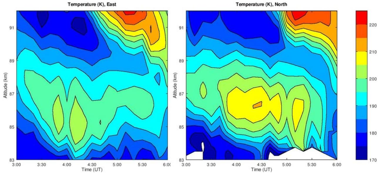
**Figure 6.** The USU Na lidar measured the time variations neutral temperature within the OH layer from east-pointing laser beam (left) and north-pointing laser beam (right) during the wave “blocking” event on the night of 11 September 2016.
