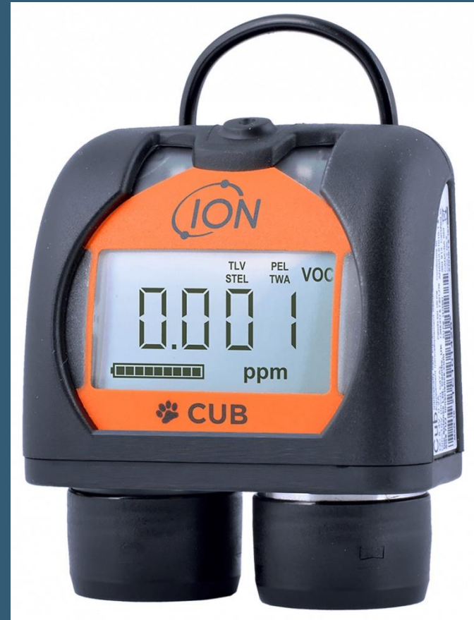
ION Cub personal VOC detector, with a 10.6 eV PID lamp and datalogger
