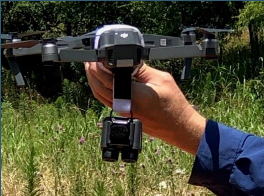
DJI Mavic Pro with Ion Cub PID attached directly below the sUAS
