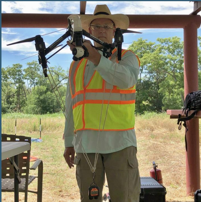
DJI Inspire 1 with Ion Cub PID attached with a short tether
