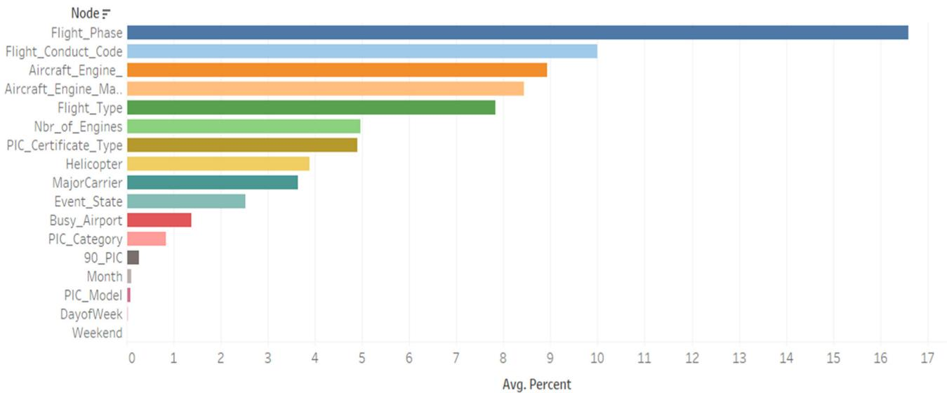
Fig. 5. Sensitivity analysis of aircraft damage-related factors.
