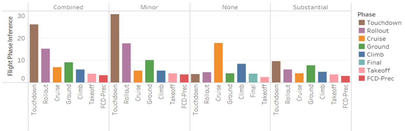
Fig. 6. Sensitivity of aircraft damage to flight phases.
