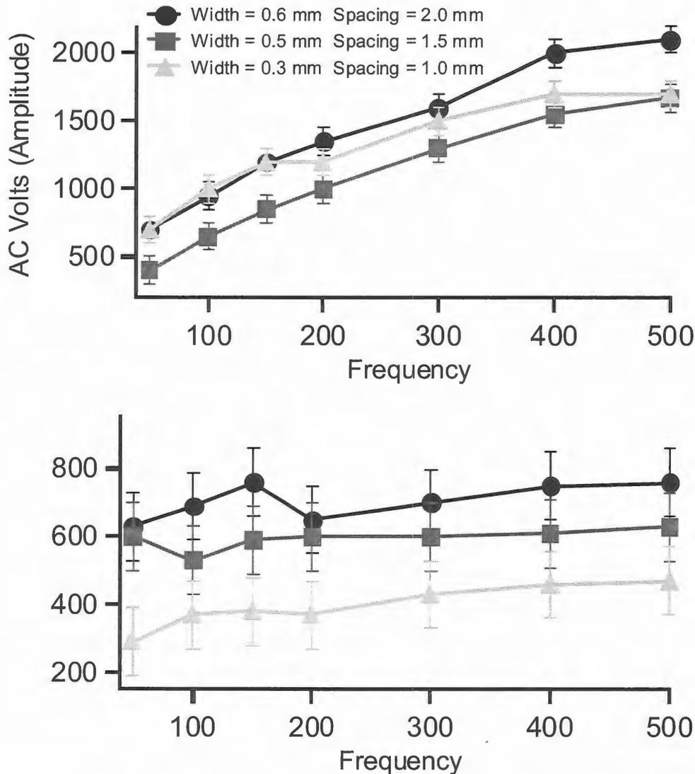
**Figure 2.** The minimum voltage required for particle transport as a function of frequency for screens of various widths and spacings at (top) atmospheric pressures and (bottom) at simulated Martian pressures 7 torr CO<sub>2</sub>.
