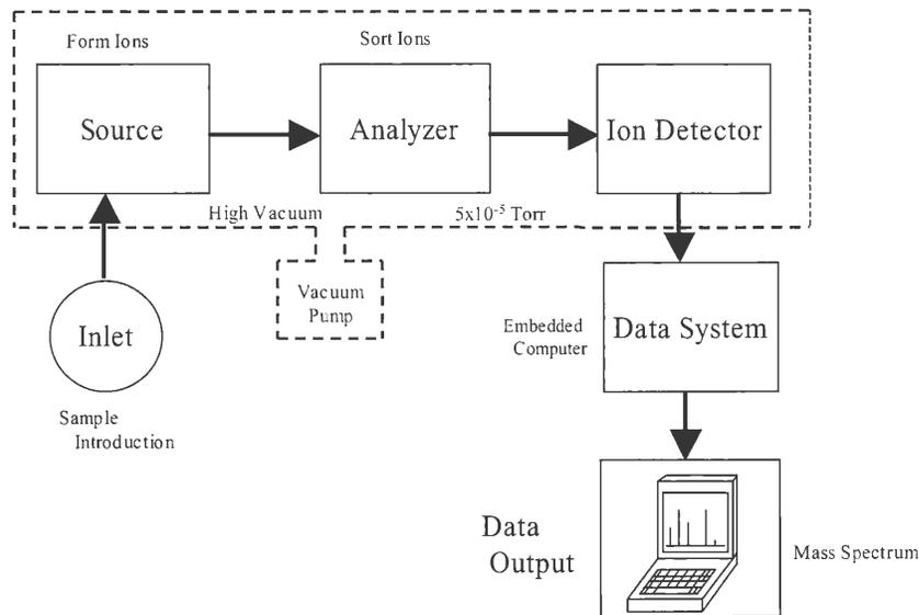
Figure 1 – A General Mass Spectrometer Block Diagram
