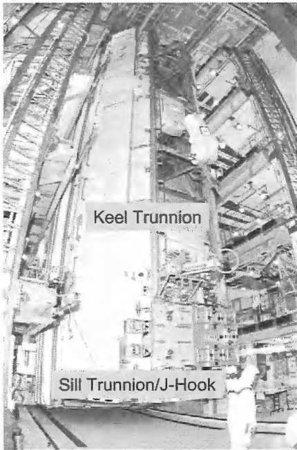
Figure 2. S-1 truss mid-transfer for STS-112.
