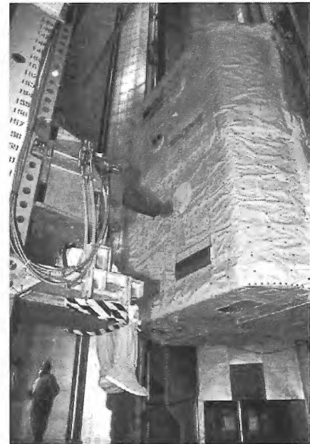
Figure 3. J-hook operator observes transfer during STS-83. The J-hook is in the center of the image.
