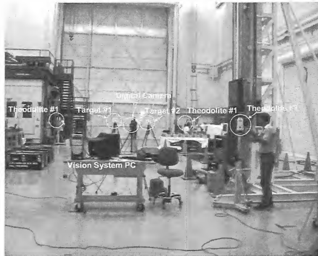
Figure 7. Camera Measurement System used in a surveying scale application.
