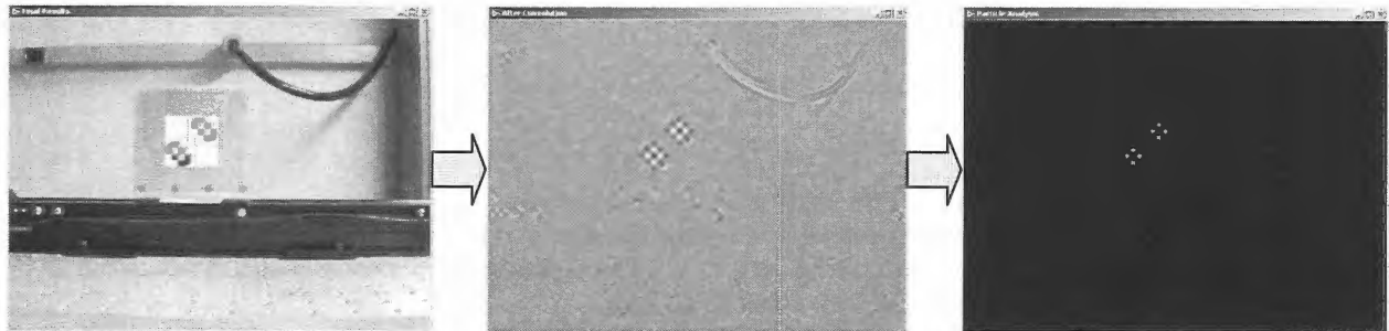
Figure 5. Images showing the novel target/convolution algorithm. The left frame shows the raw image from the camera, including the target. The center frame is the image after applying the convolution filter. The right frame is after thresholding. Notice how the target is uniquely located.
