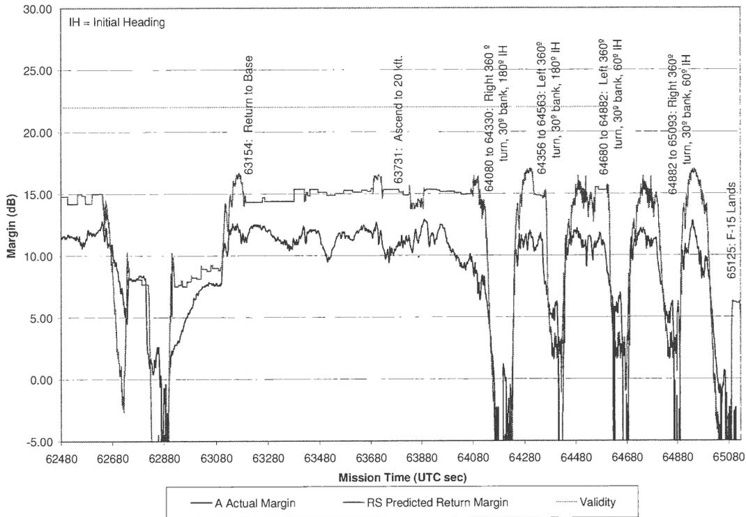
**Figure 4. Flight 6 RS Telemetry Link Margins**
