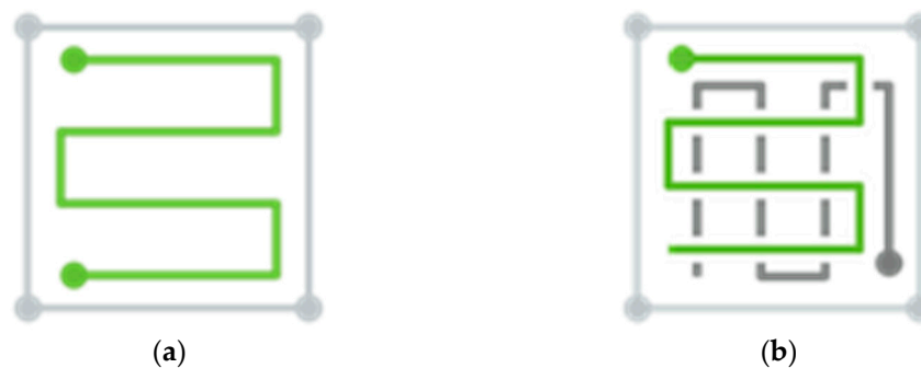
Figure 2. (a) Depiction of a single-grid flight pattern; (b) Depiction of a double-grid flight pattern.
