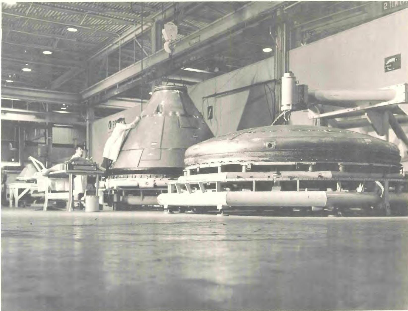
Figure 1 Stainless Steel Sections of Apollo Command Module
