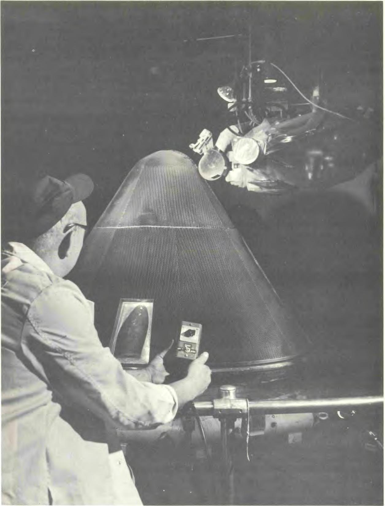
Figure 4 Machining Honeycomb
