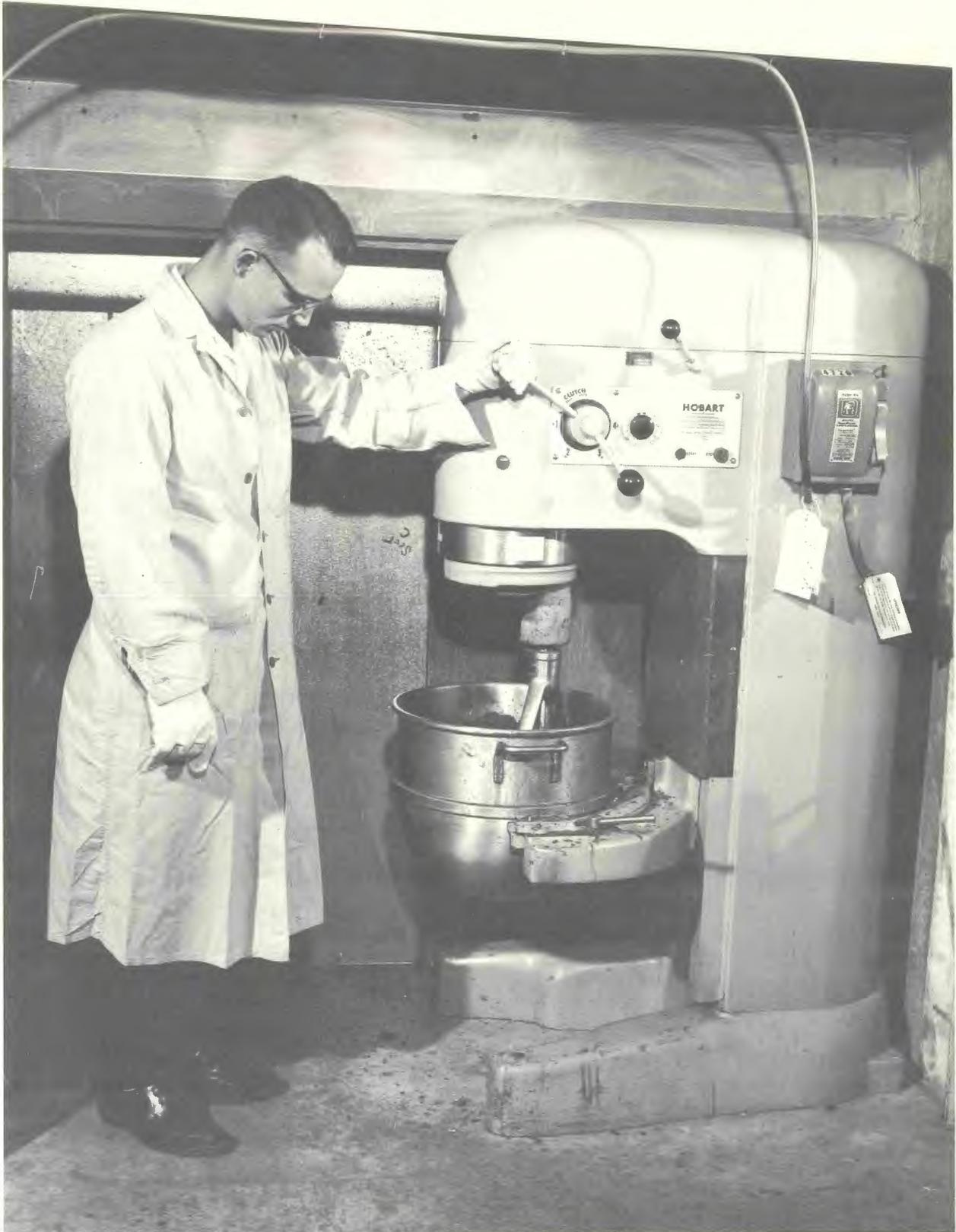
Figure 6    Mixing the Ablative Material
