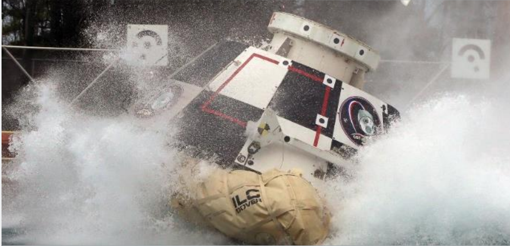
Starliner performs first contingency water drop qualification test at Langley Research Center, Virginia
