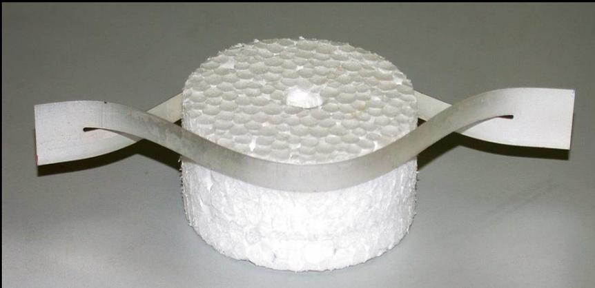
A closed loop made out of coated conductor.
