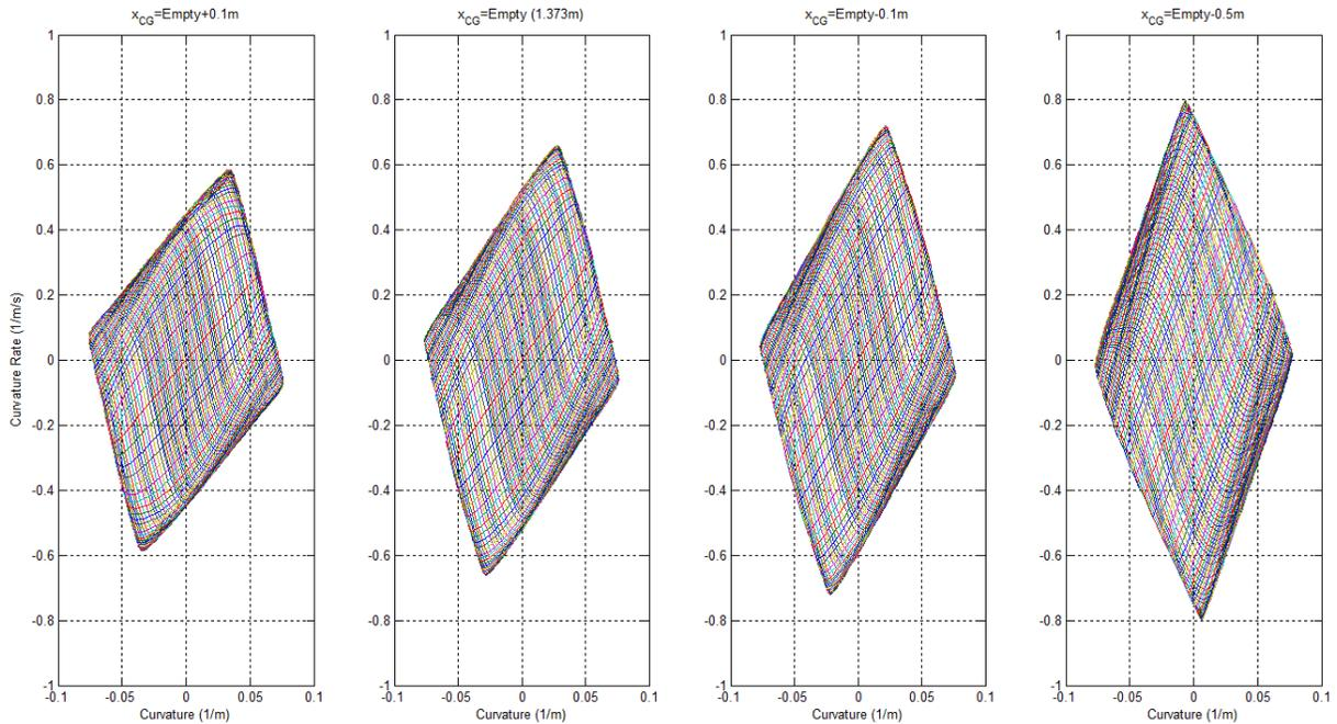
**Fig. 6:** Plot of maneuvering space diagrams showing the effect of variation of the  $x$  position of the CG. Note that the vehicle tends to oversteer (the peaks of the plot cross the curvature axis) as the CG shifts rearward.
