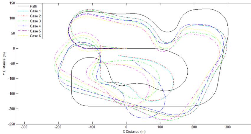
**Fig. 5:** Results of simulation using force-moment model with CG variation as given by Table 3. Note the divergence in the path tracks compared to the results of Fig. 4 as parameters are varied from nominal.
