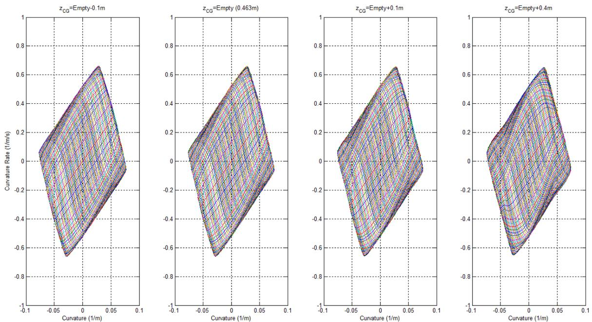
**Fig. 8:** Plot of maneuvering space diagrams showing the effect of variation of the  $z$  position of the CG. Note that the vehicle is largely insensitive to variation in this parameter in terms of maneuvering space.
