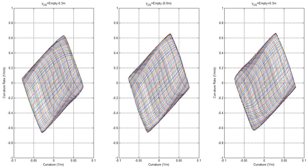
**Fig. 7:** Plot of maneuvering space diagrams showing the effect of variation of the  $y$  position of the CG. Note that the vehicle is largely insensitive to variation in this parameter in terms of maneuvering space, although some effect is seen near the upper and lower bounds of the plot.
