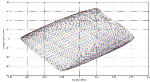
**Fig. 2:** Example of a maneuver space in terms of path curvature versus curvature rate at a constant longitudinal force across the space of front and rear slip angles. Each line with a negative slope represents a constant front wheel steering angle and each line with a positive slope indicates a constant body slip angle.
