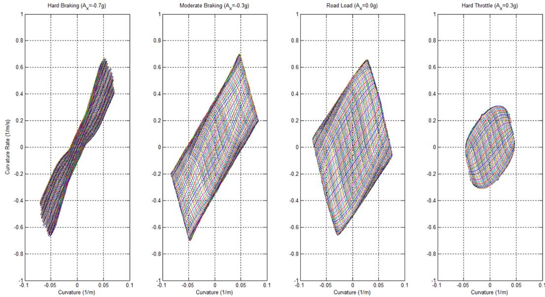
**Fig. 12:** Plot of force-moment diagrams for varying values of longitudinal acceleration. Note the dramatic difference in the size and shape of the total maneuvering space when the vehicle is at high throttle or heavy braking.
