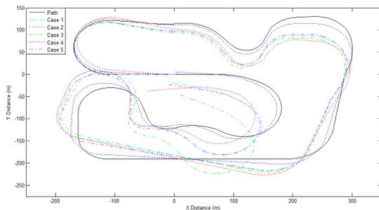
**Fig. 4:** Results of simulation using force-moment model with CG variation as given by Table 2. Note that although the simulation was run purely open loop, the desired trajectory is accurately recreated.
