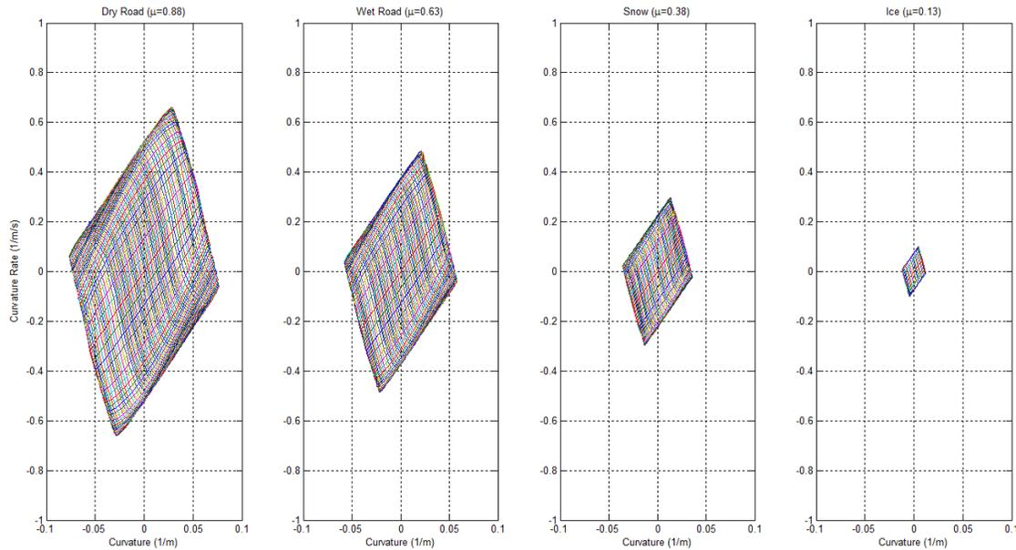
**Fig. 11:** Plot of force-moment diagrams for varying values of coefficient of friction. Note the dramatic difference in the size of the total maneuvering space and the corresponding limits of vehicle performance in terms of the motion variables.
