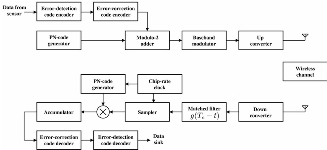
**Figure 2.** Schematic of Uplink Transmitter and Receiver
