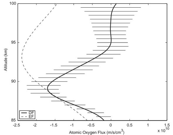
Fig. 3. Predicted dynamical (solid line) and eddy (dashed line) fluxes of atomic oxygen using Eqs. (6) and (1) with  $D_{zz} = 200 \text{ m}^2/\text{s}$  and the calculated heat flux shown in Fig. 2. Uncertainty of the dynamical flux is shown with  $1-\sigma$  error bars.
