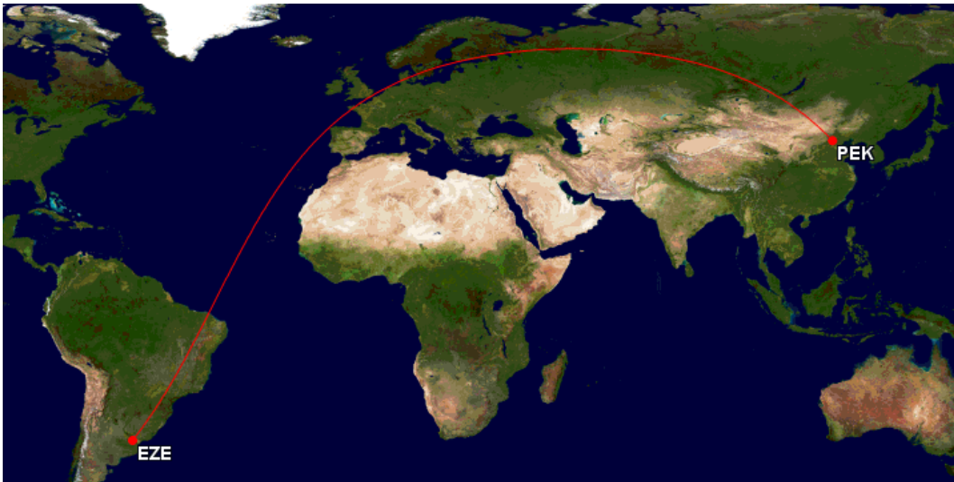
Figure 8. Great circle route EZE to PEK (10,415 NM) on conformal cylindrical Mercator chart. Courtesy of GC Mapper. Maps generated by the Great Circle Mapper ( www.gcmap.com ) - copyright © Karl L. Swartz.
