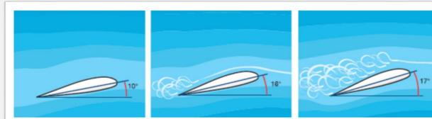
Fig. 1 – Angle of Attack<sup>1</sup>
