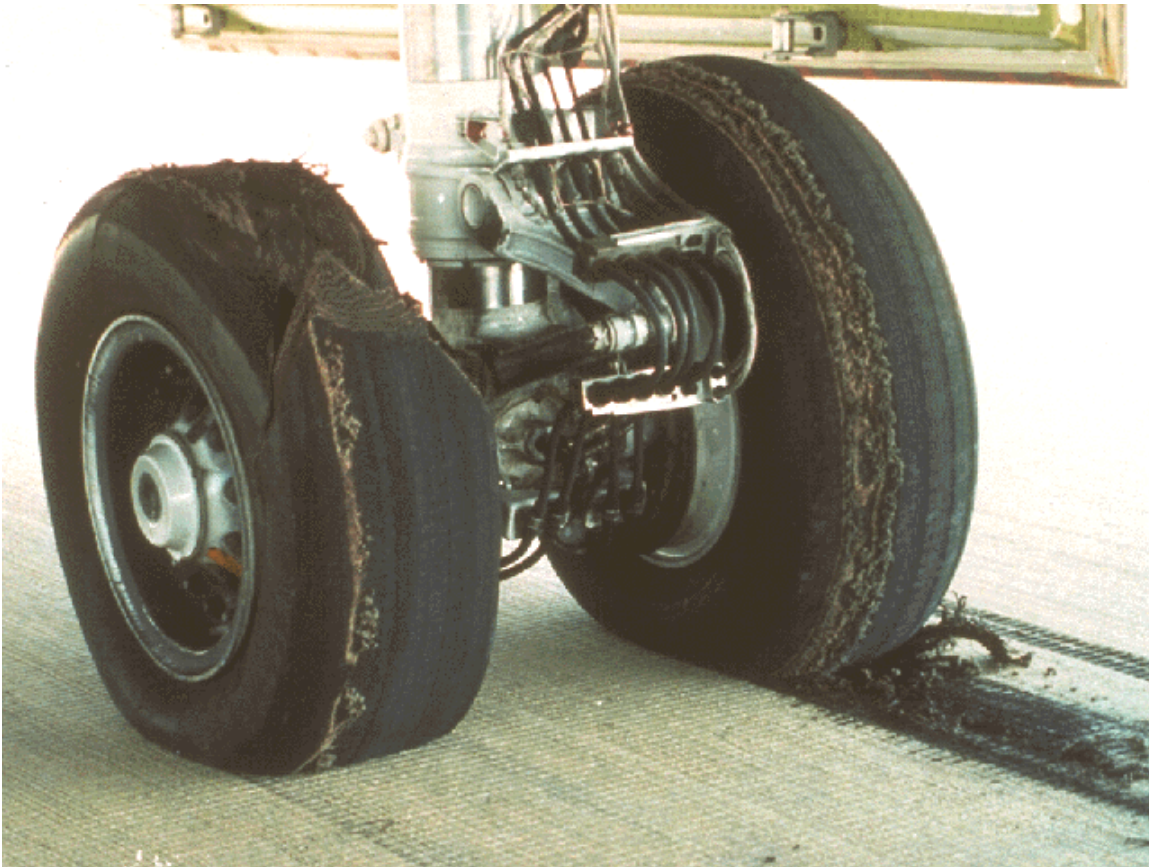
Figure 2: Orbiter Discovery experienced a blown tire during STS 51-D end of mission rollout.
