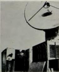
Figure 1. Shipboard SATCOM Terminal AN/SSC-3
