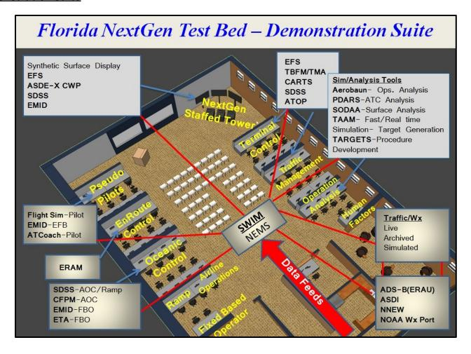
The demonstration suite is at the core of the FTB mission. It is approximately 5,000 square feet and is used to conduct demonstrations of the operational capabilities deployed at the FTB. Designed to accommodate flexibility and future growth, the suite contains reconfigurable bay areas positioned along the periphery to accommodate demonstrating and visualizing different flight domains or operational areas.
